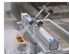
Water resistance test simulating high-pressure cleaning of power window switch
